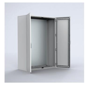
IP 55 | TYPE 12, 13 | IK 10 CE III @ KEU ₪ @ @ The mild steel double door compact floor standing enclosure range, MKD, is ideal for installation in confined spaces where a single door, when opened, would take up too much space in front of the enclosure. The doors' loading capacity also increases as it is divided over two doors. With a IP 55 protection degree, components inside the enclosure are well protected and makes it well suited for many different applications.
